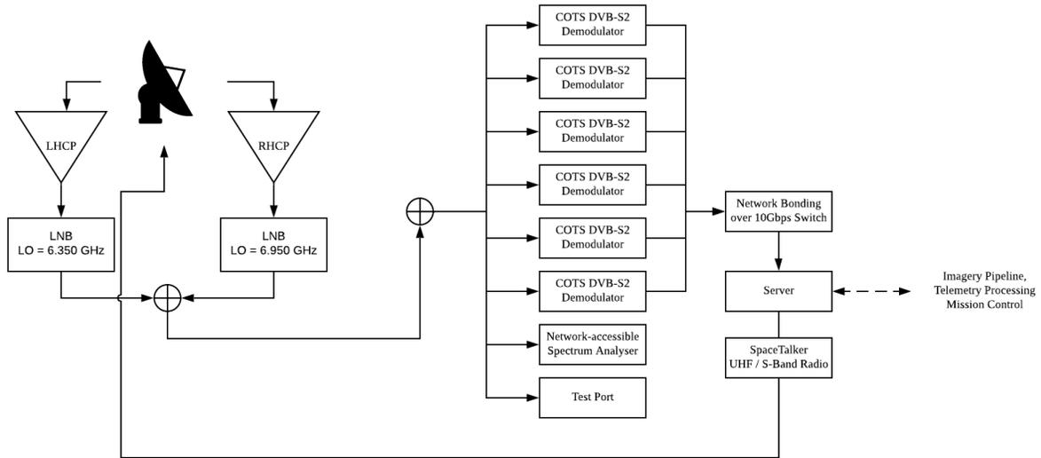
Figure 5: Block diagram of the six channel HSD2-capable ground station.
