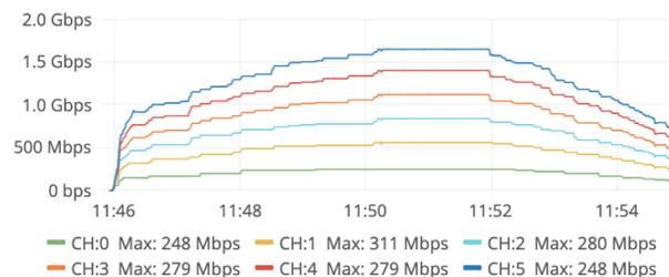
Figure 12: The data rate recorded by the demodulator shows max data rates between 248 Mbps to 311 Mbps for the six channels.
