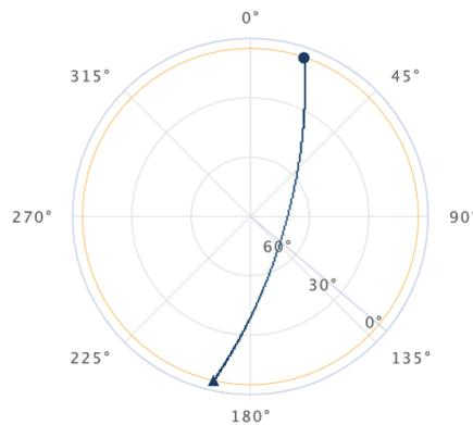
Figure 8: Azimuth and elevation angles of the satellite 2227 pass over the Keflavik ground station on May 28, 2019.
