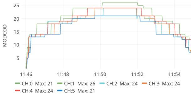
Figure 11: MODCOD is adaptively incremented or decremented based on link availability by the ACM algorithm on an individual channel basis. The modulation changes from QPSK at the start of the pass to 16/32APSK at the middle of the pass for various channels.
