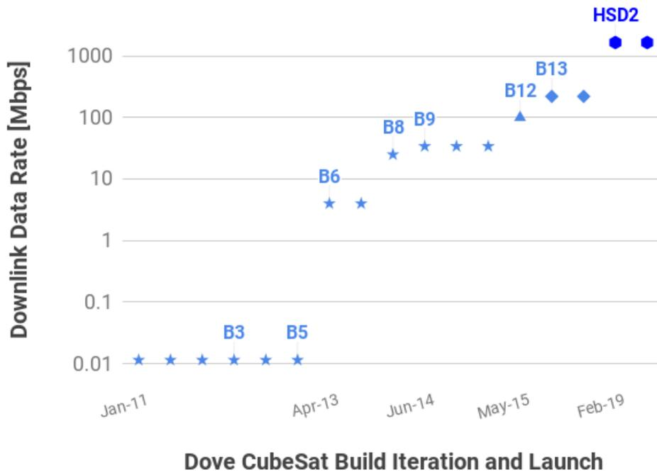
Figure 1: HSD data rate improvements for various Dove build iterations are shown as blue points on the scatter plot. Triangle represents 100 Mbps radio launched on B12 in May 2015, diamond represents the 220 Mbps radio launched on B13 in May 2016, and hexagon represents the 1.6 Gbps HSD2 radio launched in December 2018 and March 2019.
