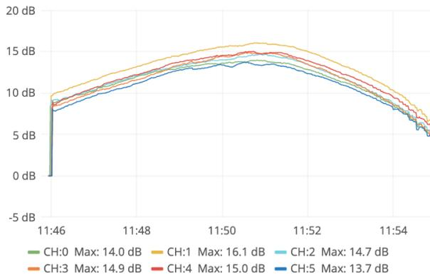
Figure 10: The demodulator recorded signal to noise ratio (SNR) is shown for the six channels at the ground station.
