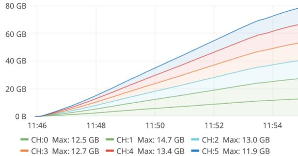
Figure 13: The cumulative data downloaded from the satellite is about 80 GB.
