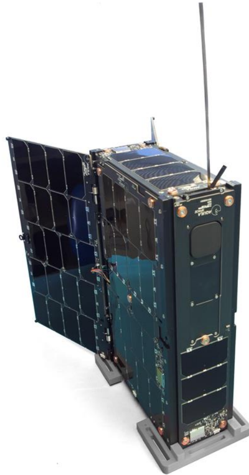
Figure 4: A view of the +X, -Z, -Y Fixed Smart Solar Panels
