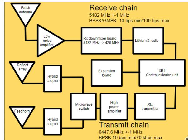
Figure 3: CU-E<sup>3</sup> Communications System Block Diagram
