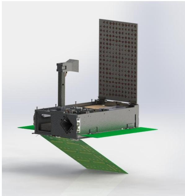
**Figure 2: Model of CU-E<sup>3</sup> cubesat with primary feedhorn/reflect array and solar cells deployed**
