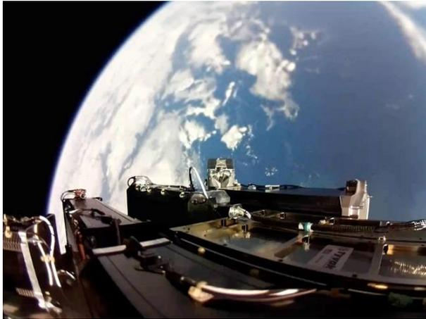
**Figure 4: Payloads mounted on Electron's Kick Stage prior to deployment, 11/11/2018.**
