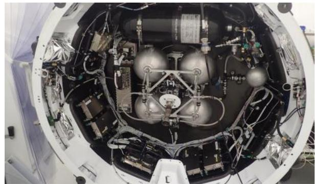
**Figure 3: Electron’s Kick Stage, including Curie Engine.**
