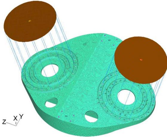
**Figure 4: Finite element model of a DPA.**
