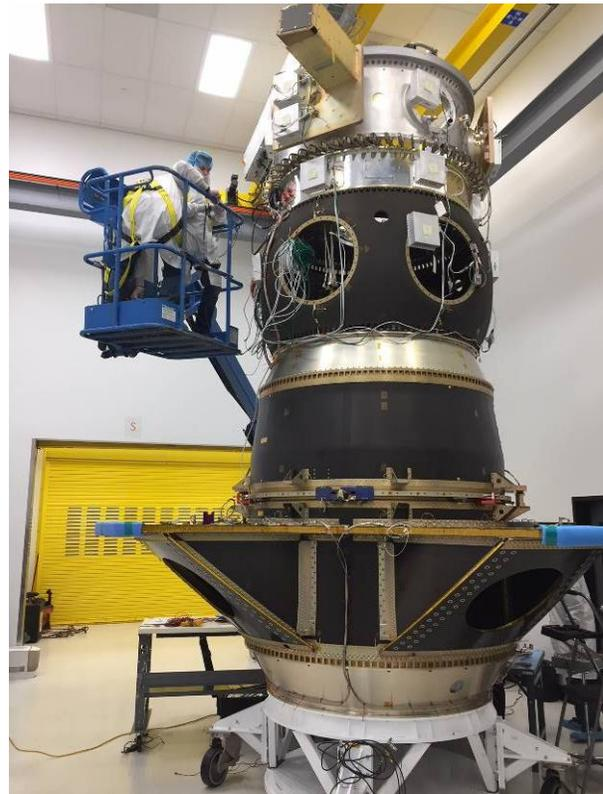
**Figure 12: Mission Director Adam Hadaller and Integration Engineer Jake Larkin prepare for a full system electrical check in Spaceflight’s Auburn Integration Facility. Note the Separation System Simulators (gray boxes) suspended by the ports to simulate spacecraft deployers.**
