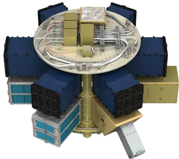
**Figure 6: Lower Free-Flyer in flight configuration. Note the two different types of dispensers, the mass model (right) that replaced an unpopulated dispenser, and the DragSail (silver object to the lower right). The avionics system is on top.**
