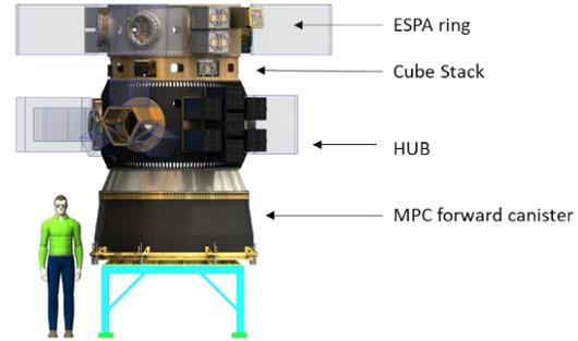
**Figure 3: Upper Free-Flyer Configuration.** Note that the MPC forward canister is bolted to the HUB above, and connected via a clampband separation system to the MPC lower canister.
