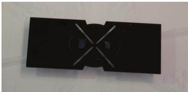
**Figure 4: Prototype of the silicon MEMS gravity gradiometer**
