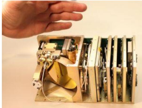
**Figure 2: Fibertek's Compact Laser Communications Terminal.**
