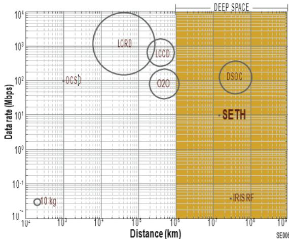
**Figure 1: Comparison of SETH capability with that of the other NASA optical communication activities and IRIS Radio Frequency (RF) system. Circle size indicates flight terminal mass.**
