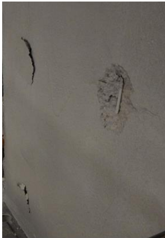
Figure 4-30 Punch through observed in all 3-in. specimens with Connector C
