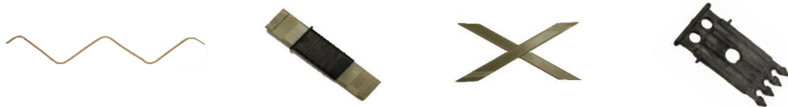
Figure 3-25 Shear Connectors Tested, Left to Right: Connector A, B, C, and D
