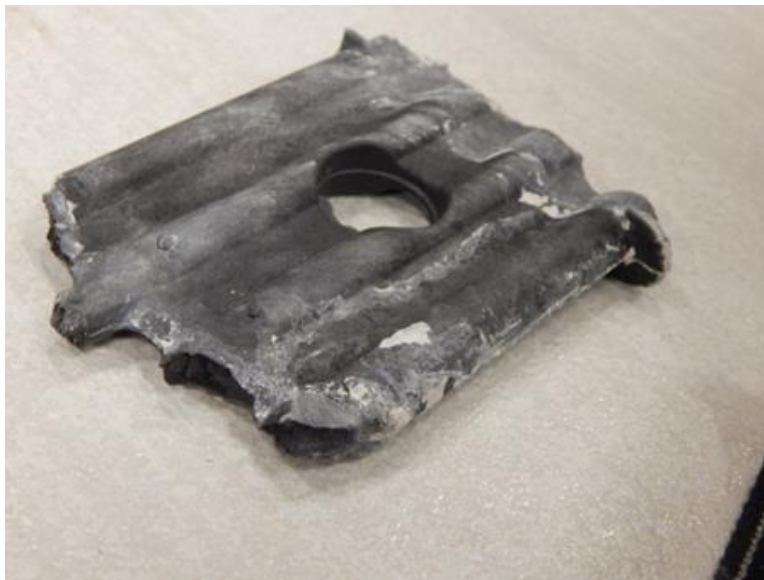
Figure 4-33 Shear fracture of Connector D, both ends fractured
