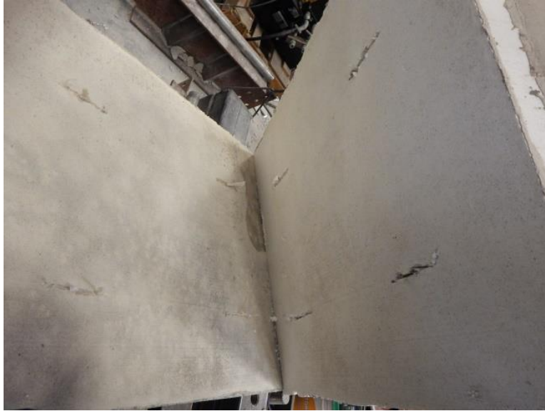
Figure 4-35 Three inch bonded EPS connector E tensile rupture of all connectors
