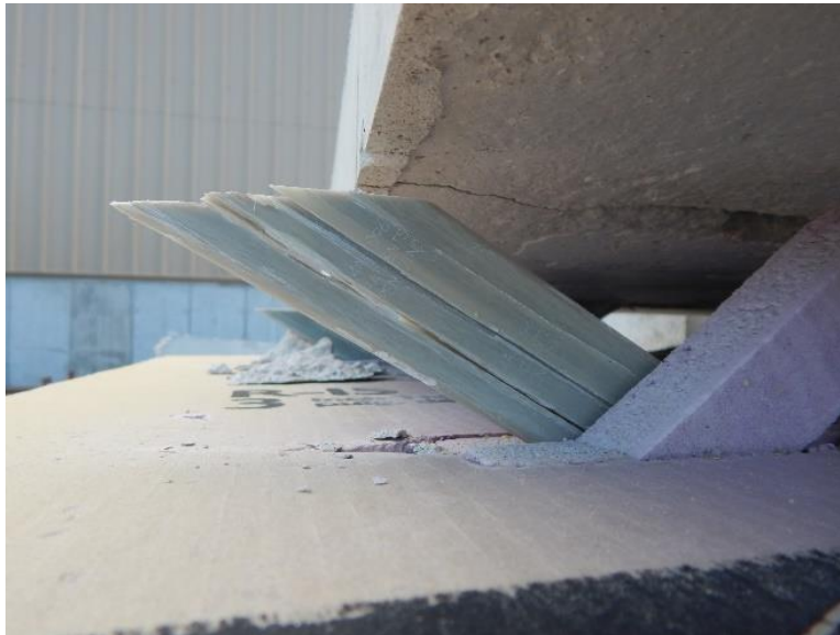
Figure 4-28 Delamination / shear rupture in a 4-in. bonded XPS specimen
