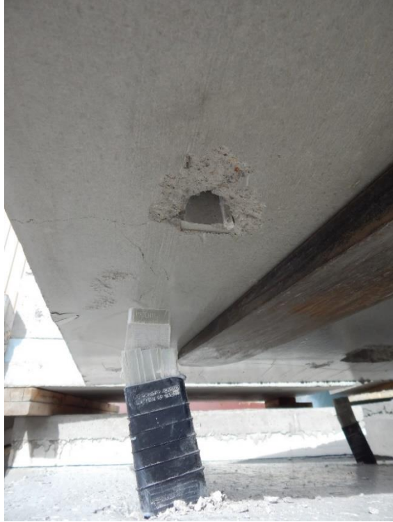
Figure 4-24 Pullout occurring with Connector B in combination with bending fracture
