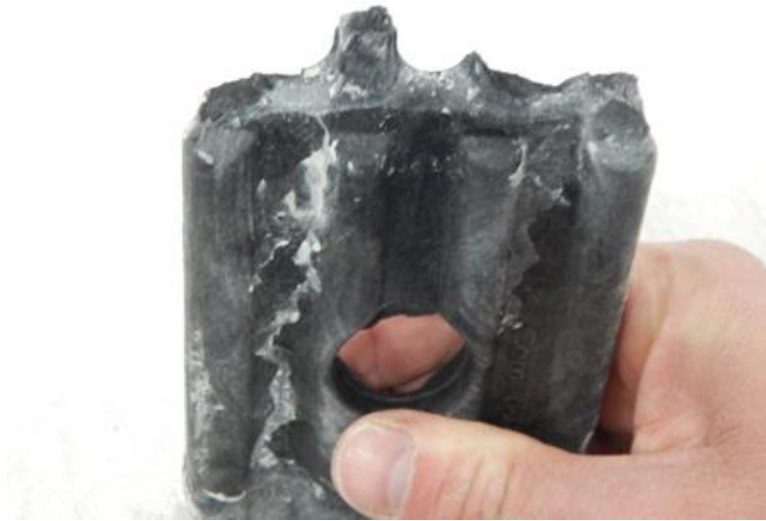
Figure 4-34 Close-up of shear fracture of connector D
