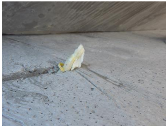
Figure 4-17 Tensile rupture in unbonded specimen with ISO foam
