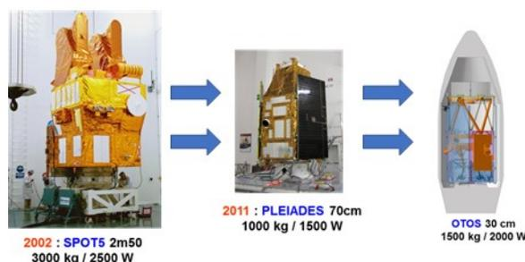
**Figure 1: Example of payload miniaturization for Earth Observation missions**
