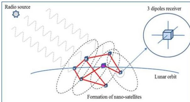
Figure 4: Satellite NOIRE network configuration
