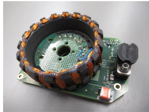
**Figure 3: Reaction wheel electronics assembly**
