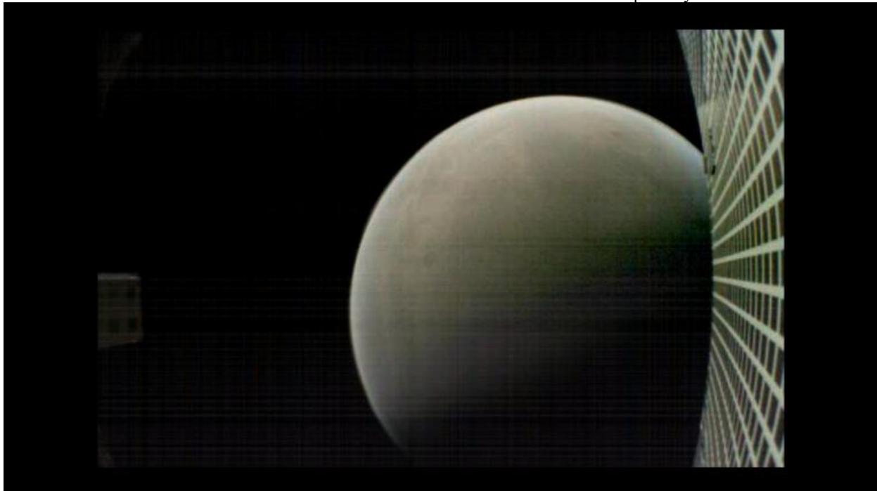
**Figure 6: Mars, as imaged by MarCO-B, just following InSight's entry-descent-and-landing. The right hand side of the image shows the high gain reflectarray, while the left has the high-gain feed. The image was taken by MarCO-B's wide-field-of-view camera.**
