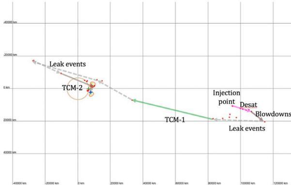
**Figure 3: MarCO-B path to Mars (TCM's 1 & 2). Mars is shown by the circle on the left. The small contours represent the best trajectory for relay at a specific point of time as shown in the B-plane.**
