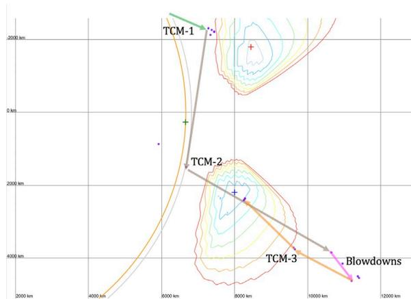
**Figure 2: MarCO-A path to Mars, including TCM-1, TCM-2, and TCM-3. Mars is shown by the circle on the left. The contours represent the best trajectory for relay at a specific point of time as shown in the B-plane.**
