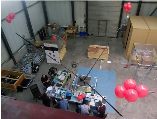
Figure 9: Fully deployed antennas
