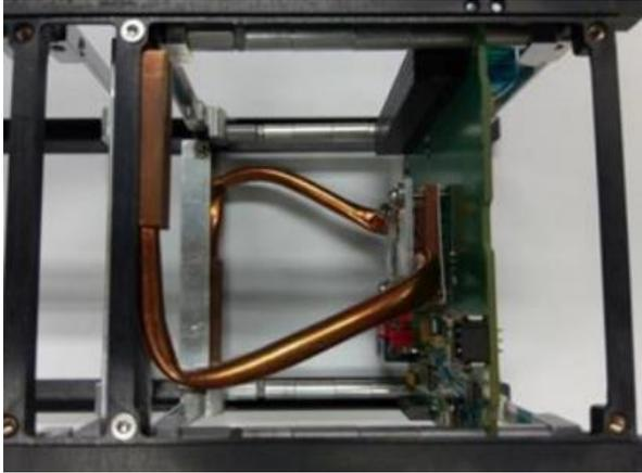
**Figure 2: ISIS' CubeSat Heat Pipe**
