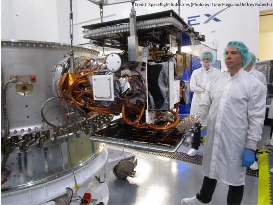
Figure 5: STPSat-5 Horizontal Integration to Launch Stack
