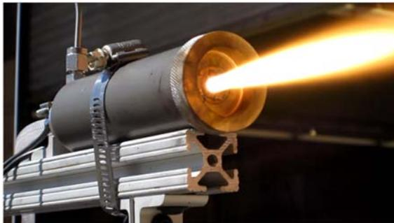
**Figure 4: 25-N High Performance Green Hybrid Propulsion System During Test Firing Sequence.**
