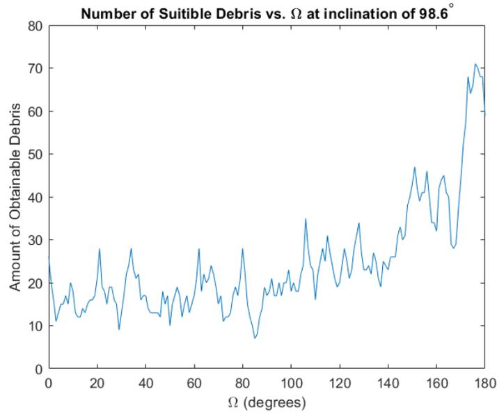
Figure 4: Number of suitable pieces of debris vs. right ascension of ascending node ( $i = 98.6^\circ$ )
