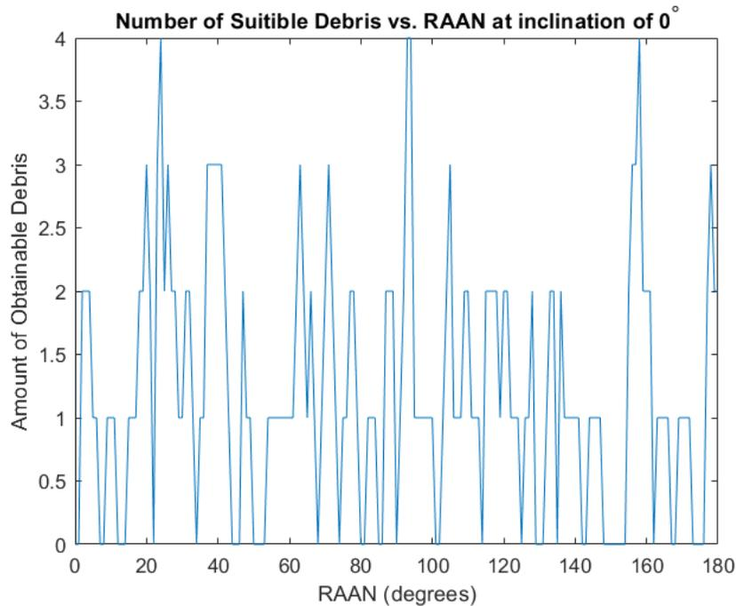
Figure 5: Number of suitable pieces of debris vs. right ascension of ascending node ( $i = 0^\circ$ )
