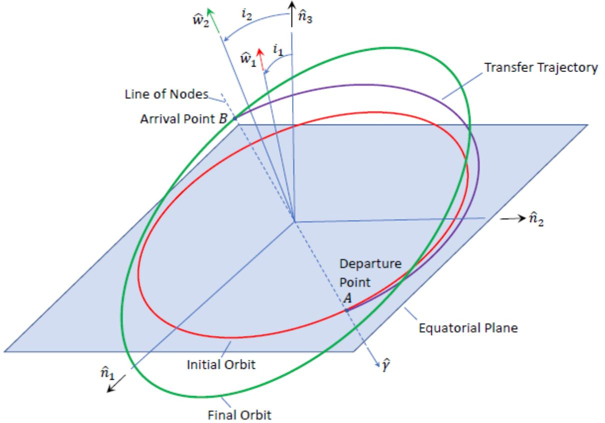
Figure 1: Inclined orbit, showing relevant unit vectors and angles
