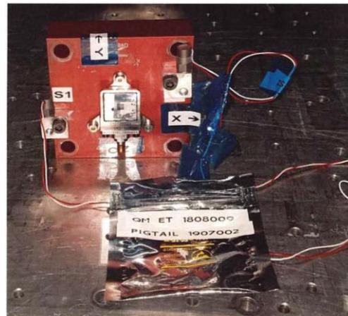
**Figure 19: Pyro shock test setup Y axis**
