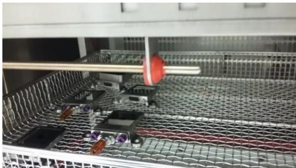
**Figure 21: Sensors in thermal shock chamber**
