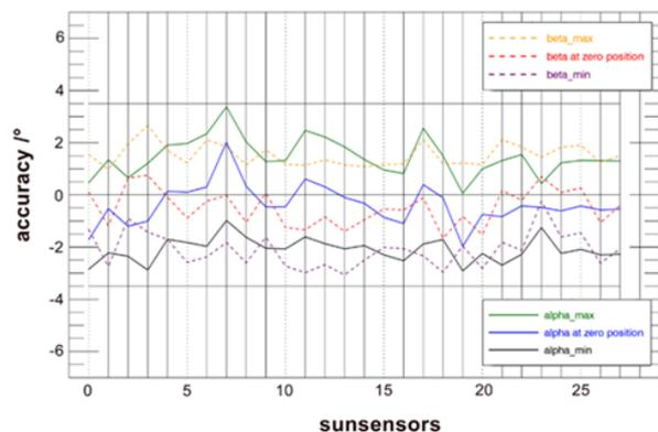
**Figure 7: non-calibrated accuracy for manual assembly**
