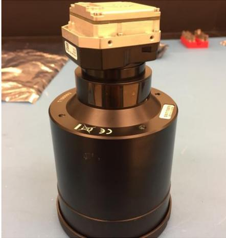
**Figure 3: Tau 2 640 Infrared Imager and Lens**
