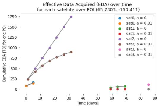
Figure 7: Cumulative EDA for one POI for each of the 4 satellites, with  $a = 0$ , for no sensor degradation over time and  $a = 0.01$ , an extreme case of sensor degradation of 1 % / day.
