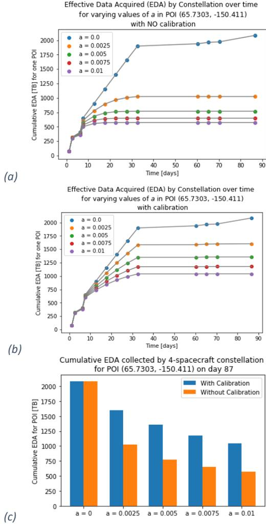
Figure 6: EDA for one Point of Interest (POI) for the constellation. 6a shows the case without calibration, and 6b is the case with calibration. 6c compares the cumulative EDA collected by day 87, for both the calibration (blue) and no-calibration (orange) case.
