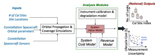
Figure 2: CalVIN consists of modules for computing calibration system costs and value for EO missions.
