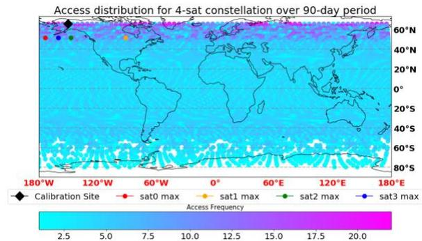
Figure 5: Points of Interest within a global Region of Interest (ROI), with the constraint of latitudes  $< 66.5^\circ$ . The color corresponds to access frequency by constellation. The dots with labels are the points associated with maximum access by each of the satellites. The black diamond was chosen as the calibration site for the constellation.
