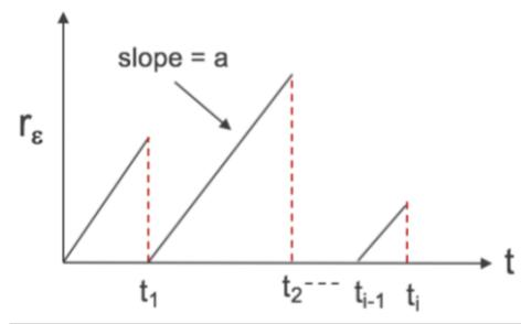
Figure 1: A stylized diagram showing how  $r_\epsilon$ , that quantifies data degradation due to loss of sensor calibration, may vary over time with calibration events occurring at time instances  $t_i$ . Each calibration event resets this data degradation factor to zero. The calibration events may not be spaced equally in time due to the specifics of the orbital geometry and the location of the calibration site.
