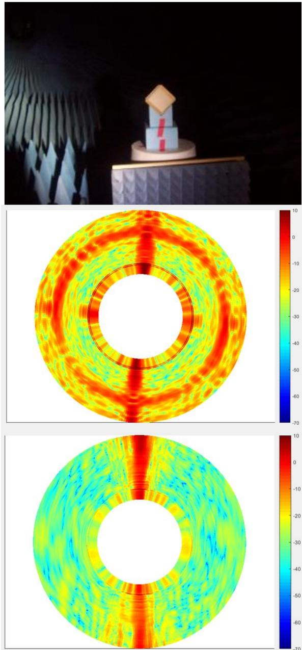
**Figure 6: Radar cross section measurements of 1U cube oriented so it rotates face to edge to face in the vertical axis (top). RCS vs. frequency (in radial axis) and angle measurements with NTE retro-reflectors (middle) and without (bottom).**
