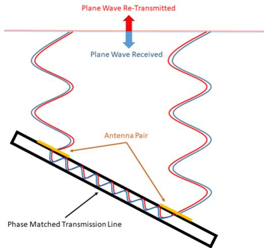
**Figure 2: Phase matched transmission lines between paired antenna elements are used to propagate a reflected wave in the same direction from which it was received.**
