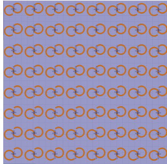
**Figure 3: FEM model of a 64-element Van Atta Array used in the Nanosat Tracking Experiment (NTE) devices.**
