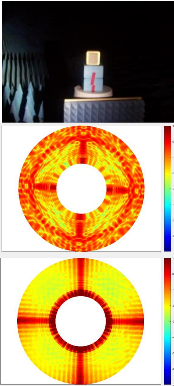
**Figure 5: Radar cross section measurements of a 1U cube oriented so it rotates from face to face in the vertical axis (top). RCS measurement vs. frequency (in radial axis) and angle with NTE retro-reflectors (middle) and without (bottom).**
