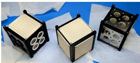
**Figure 8:** Final fabricated STAR-3 satellites with radar and optical retro-reflectors.
