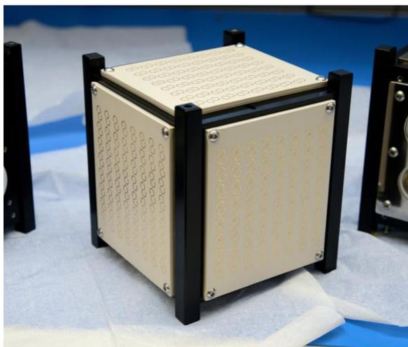
**Figure 7:** 1U STAR-3 cubesat with NTE retro-reflector panels.
