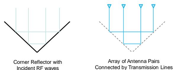
**Figure 1: A corner reflector (left) and a Van Atta Array Retro-reflector (right).**
