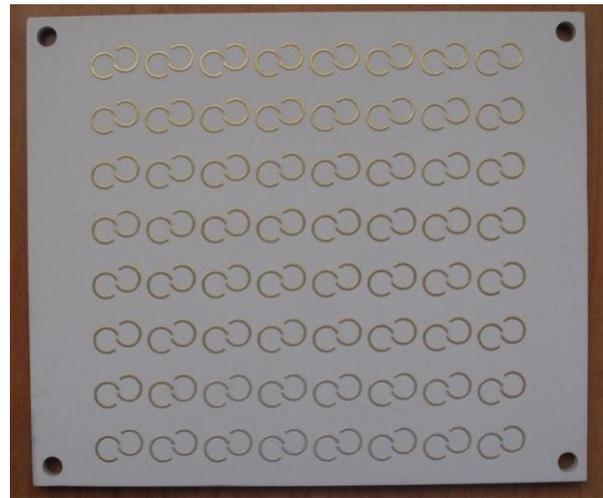
**Figure 4: A fabricated 8 x 8 NTE Van Atta Array in 1U form-factor operating in Ku-band.**
