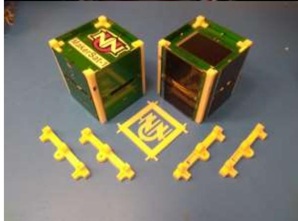
Figure 6: MakerSat-1 3D printed frame components aboard ISS
