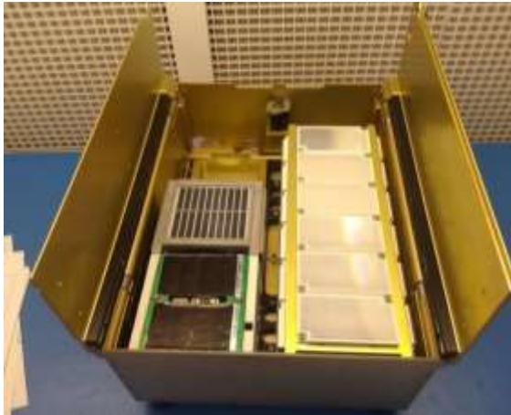
Figure 7: MakerSat-1 (lower left) loaded in Slingshot deployer
