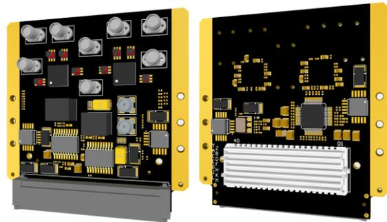
Figure 2: SDR PCB with Primary on Left and Secondary on Right
