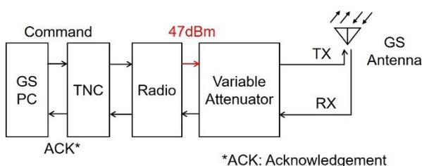
**Figure 10: GS Setup for Uplink with Radio**
