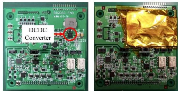
**Figure 7: Shielded DCDC Converter of FAB**
