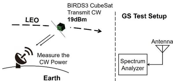
**Figure 13: Setup of the CW Measurement Test**
