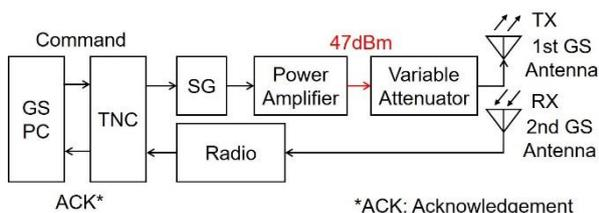
**Figure 9: GS Setup for Uplink with SG and Power Amplifier**
