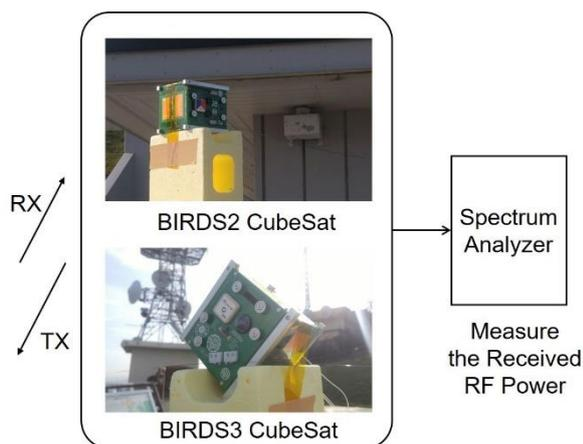
**Figure 11: CubeSat Setup at Top of the Mountain**
