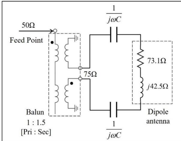
**Figure 4: Impedance Matching Circuit**
