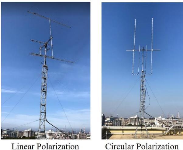
**Figure 8: Linear and Circular Polarization Antenna**
