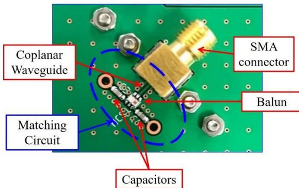
**Figure 5: Coplanar Waveguide and Matching Circuit**
