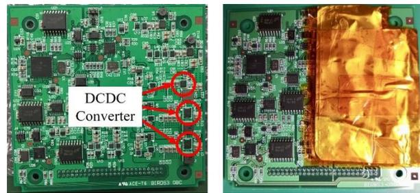
**Figure 6: Shielded DCDC Converter of OBC/EPS Board**
