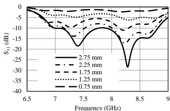
**Figure 8:  $S_{11}$  Versus Frequency for Different Probe Feed Locations (All Distances are Calculated from the Center Point of the Driven Patch)**
