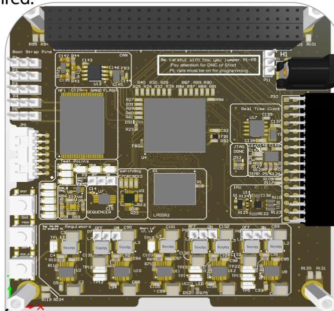
Figure 2: Render of the custom Secondary On-Board Computer for the McMaster NEUDOSE mission.
