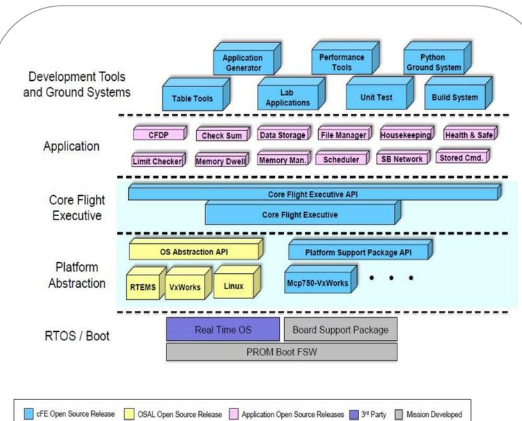
Figure 3: Software Architecture of NASA's core Flight System which is being used to develop mission-specific applications [2].
