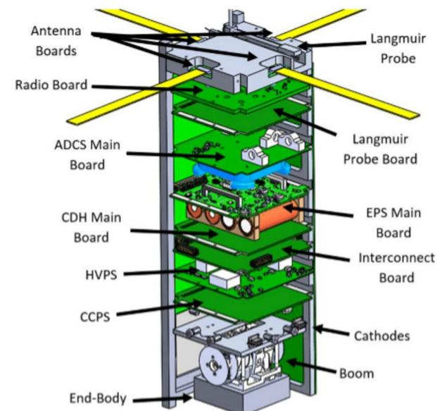
CAD image of the internal MiTEE-1 structure with labelled components.
