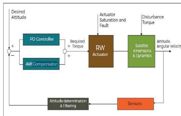
Figure: Proposed Fault-Tolerant Control Method
