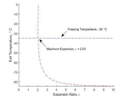
Figure 2. Maximum expansion ratio to prevent freezing
