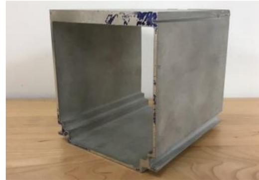
Figure 3: Waterjet cutting failure with uneven dimensions
