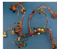
Figure 3: SFL NorSat-1 Harness with scale
