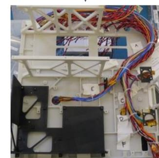
Figure 13: Author built first interstitial harness on 3D printed jig
