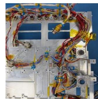
Figure 15: Final flight build interstitial harness mounted on flight structure
