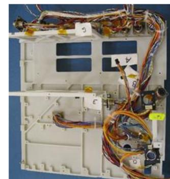
Figure 14: Technician terminated interstitial harness
