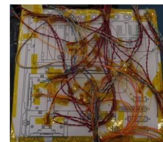
Figure 12: First attempt of cardboard routing to determine bulkhead locations
