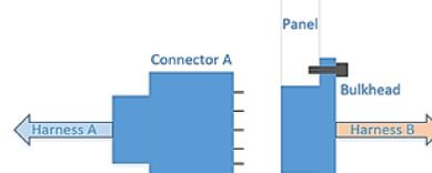
Figure 7: Bulkhead connector diagram
