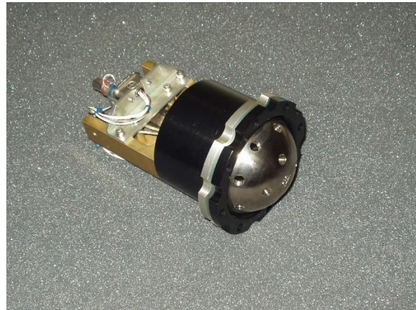
Figure 4: Starshine 5 shown stowed in its deployer.
