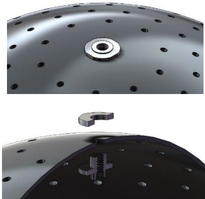
Figure 13: Starshine 4 field repair.
