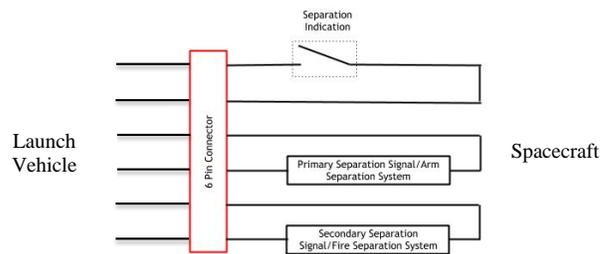
**Figure 2: SSDS Electrical Interface Circuit Diagram<sup>2</sup>**
