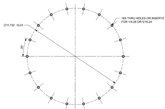
**Figure 3: Standard Class 1 Mechanical Interface<sup>2</sup>**
