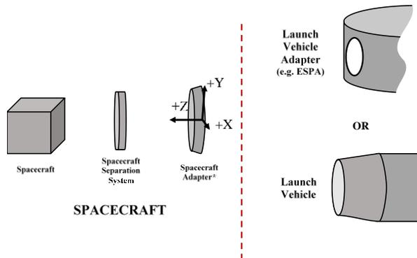
**Figure 1: Spacecraft vs Launch Vehicle Disambiguation and Coordinate System<sup>2</sup>**
