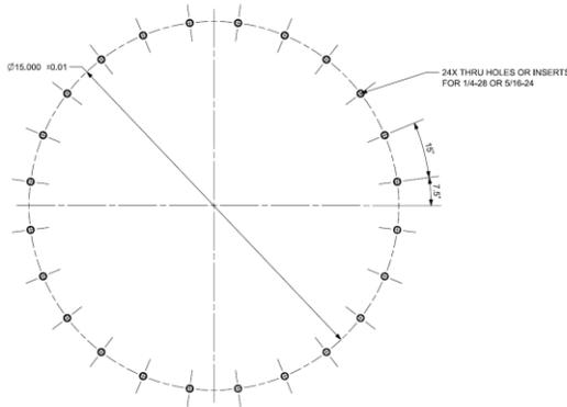
**Figure 5: Standard Class 2 and 3 Mechanical Interface<sup>2</sup>**
