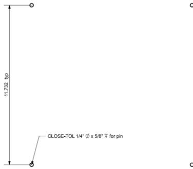
**Figure 4: Standard Class 1 4-Point Mechanical Interface<sup>2</sup>**
