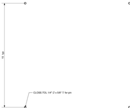
**Figure 6: Standard Class 2 and 3 4-Point Mechanical Interface<sup>2</sup>**
