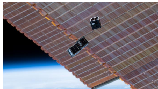
Figure 2. The Virginia Cubesat Constellation cubesats seconds after deployment from the International Space Station.
