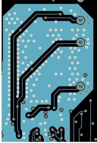
**Figure 9: Clock Via Shielding and Flood Fill**
