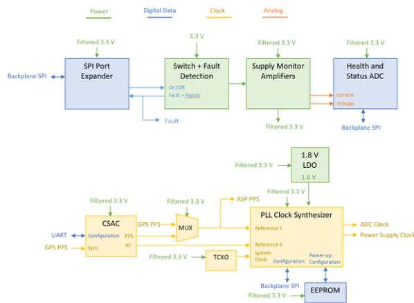
**Figure 6: Clock Board Block Diagram**
