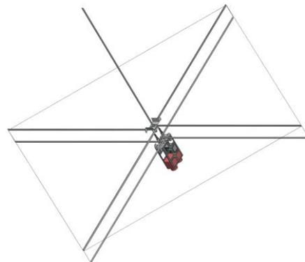
**Figure 1: Spacecraft Bus with Deployed Vector Sensor Antennae**
