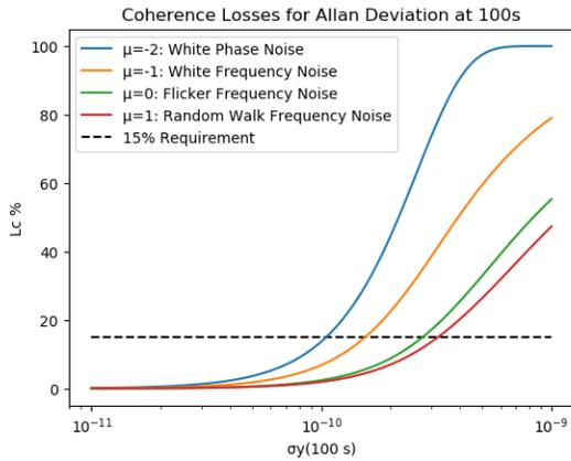
**Figure 3: Coherence Loss Allan Deviation Dependence**
