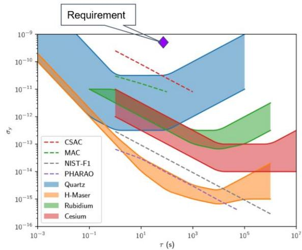
**Figure 5: Typical Reference Clock Sources<sup>9</sup>**
