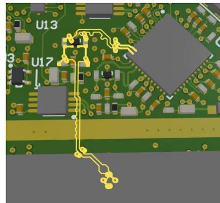
**Figure 8: ADC Reference Clock Route**
