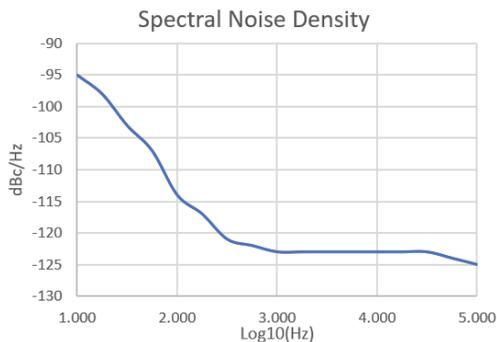
**Figure 13: CSAC with PLL Phase Noise**
