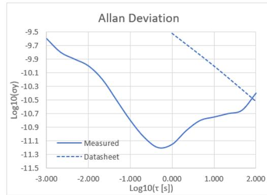
**Figure 11: CSAC with PLL Allan Deviation**
