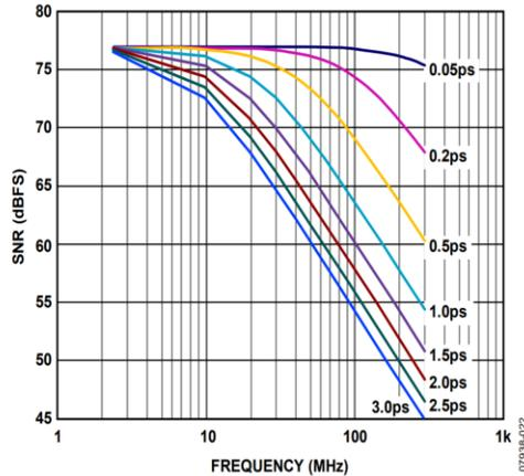
**Figure 4: ADC Clock Jitter Impact on SNR<sup>11</sup>**
