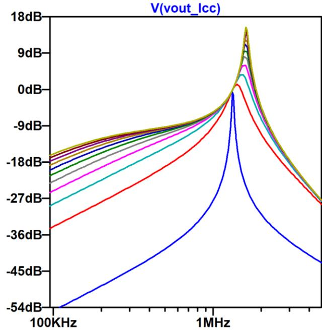
Figure 2: LCC Resonant Tank Gain Curve
