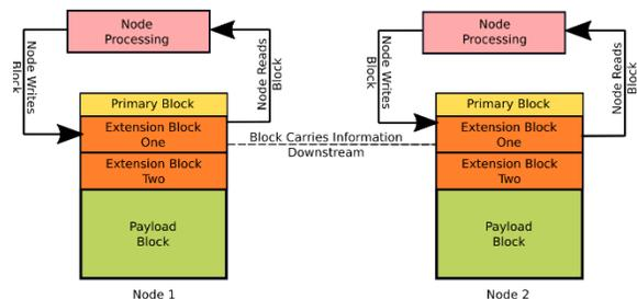
**Figure 3 - BP provides a more featureful extension header mechanism than IPv6<sup>5</sup>.**
