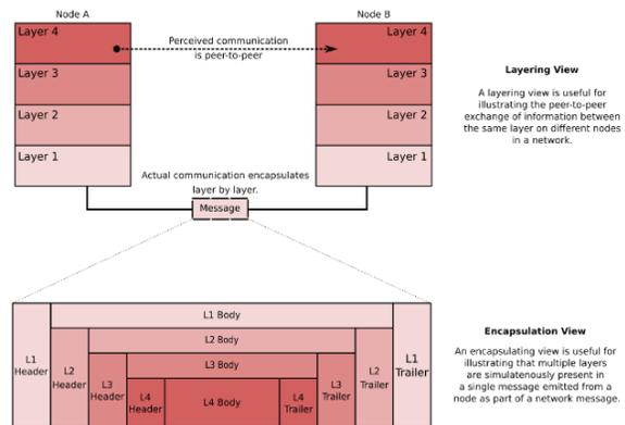
**Figure 1 - Layering is typically implemented using encapsulation<sup>5</sup>.**
