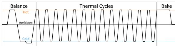
Figure 2 – Standard Thermal Vacuum Test Campaign
