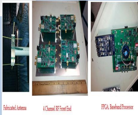
Fig 3 4 Channel VHF receiver hardware
