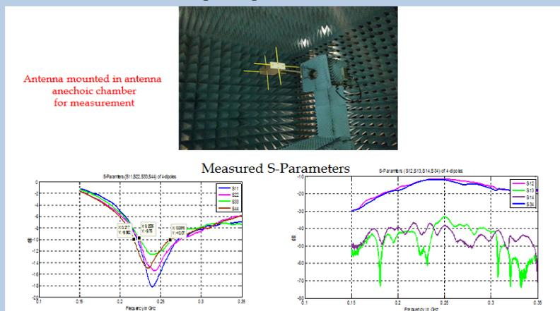
Fig 4. VHF antenna radiation patterns and input VSWR measurement results
