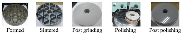
Figure 3: φ270mm F-molding ceramic at each process stage.
