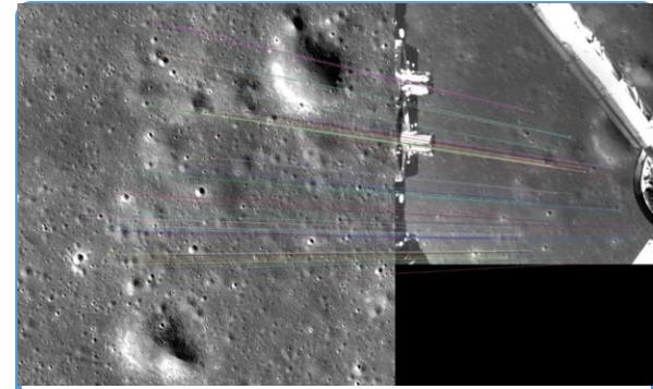
Visualization of feature extraction and matching component of terrain relative navigation on lunar imagery. The image on the right shows a subset of the lunar surface from the left image. Matched features between the images are shown connected by colored lines. Testing has also included datasets from previous sensor demonstration flights on a Masten Xombie vertical takeoff vertical landing vehicle.
