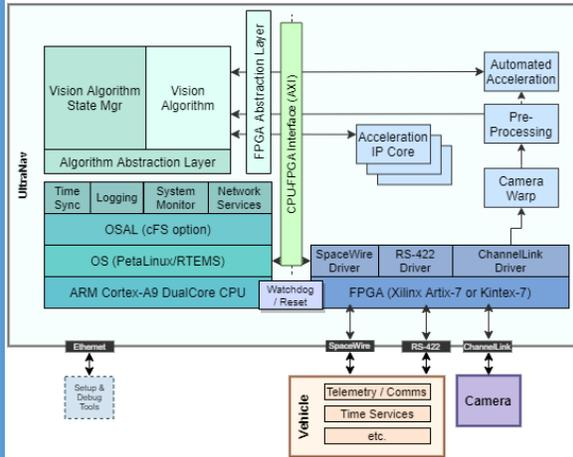
The UltraNav platform will separate vision algorithm functionality between the processor subsystem and the FPGA subsystem. Much of the infrastructure chosen to support this (e.g., PetaLinux, AXI interfaces) is open source, decreasing cost and development times.
