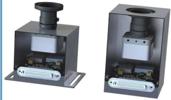
The UltraNav platform is composed of a camera (with optics) and a compute element that runs machine vision algorithms. Together, this hardware takes up a volume of approximately 1.5U. Two different enclosure options are under investigation.
