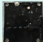
③ GROWTH board • To control the system • Originally developed for thundercloud gamma-ray detection • FPGA: Artix-7
