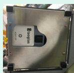
① Front cover plate • 1.6 mm thick aluminum plate
