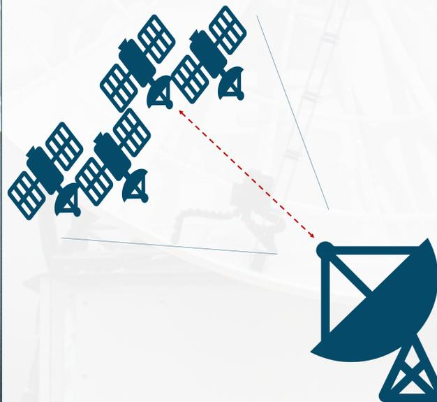
Spacecraft clusters allow multiple Ground Station contacts in the same cluster visibility window, i.e. more than one spacecraft is in the field of view of the antenna. With standard operations one visibility window can be used to communicate with just one spacecraft, thus reducing the total communication availability for the overall cluster by a factor of four (assuming same GS capacity).
