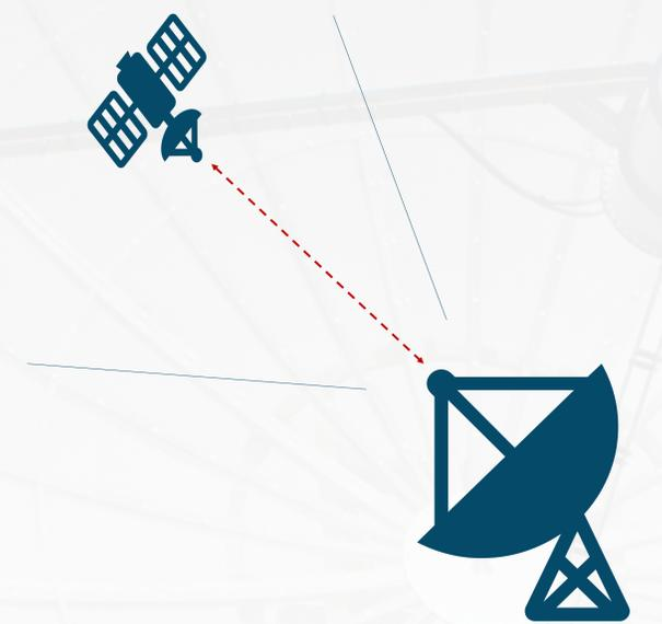
On a typical mission one GS talks with one satellite at a time during a "visibility window" when the spacecraft is in view of the GS.
