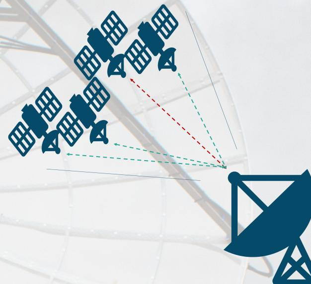
Leaf Space supports the KSM1 through the multi-mission Ground Station as a Service (GSaaS) network solution called Leaf Line. The GSaaS exploits the opportunity to maximize the contact time with each spacecraft of the cluster using the Multi Spacecraft Per Aperture (MSPA) technique.
