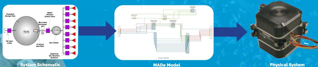
MADe fits in the product life-cycle in the design phase but can also be used for legacy systems (i.e., systems already in operation). The system concept will be developed and iterated within MADe using blocks, functions and flows to arrive at a final design supported by the different analyses (such as Fault Tree, FMEA, Reliability etc) available in the software.
