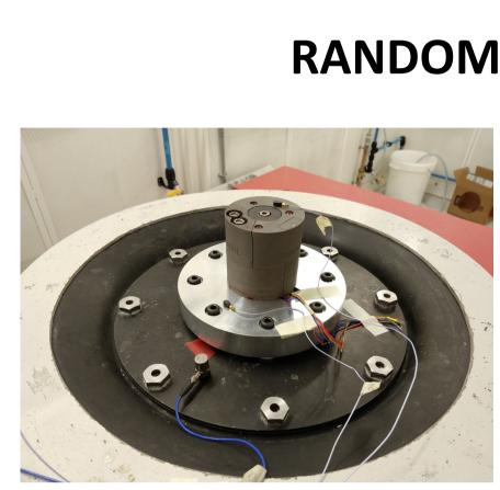
The test environments selected for the qualification campaign consisted of two levels of random vibration as reported in the tables below. The test item was subjected to each of these random vibration environments in each orthogonal axes amounting to six individual random vibration tests. A modal survey was performed before and after each test run to verify possible structural changes.
