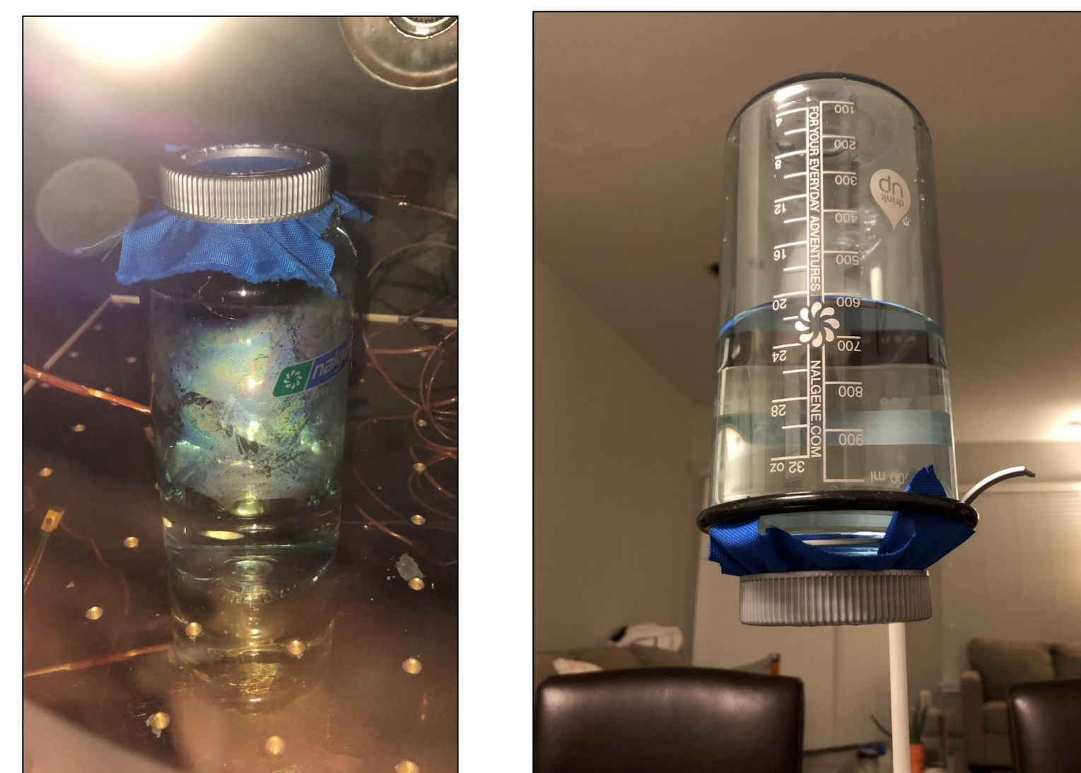
Figure 3. ePTFE material as phase separator being tested in vacuum chamber (left), and also in ambient condition (right).
