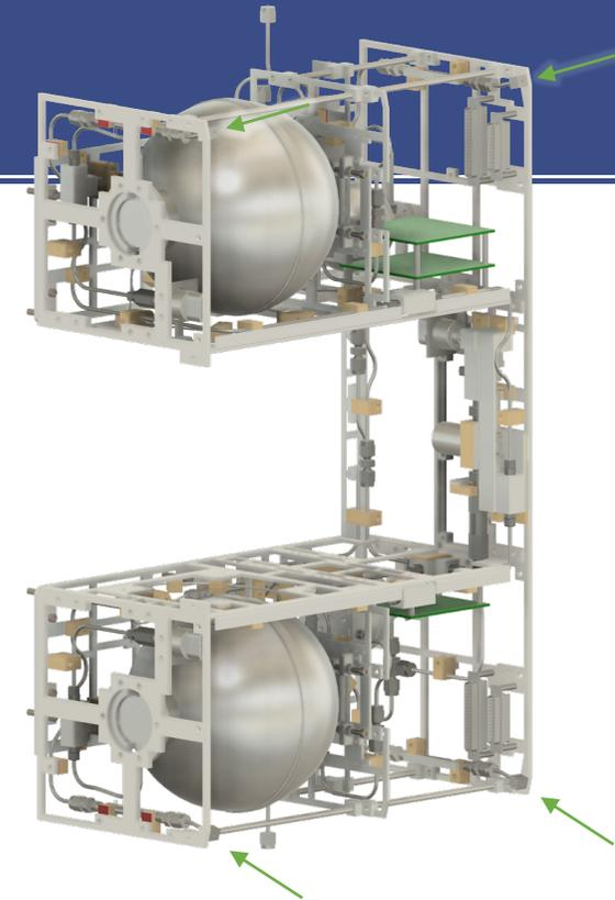
Figure 2: 3D render of ALEx propulsion unit delivered to ALE2 spacecraft. Green arrows represent forces generated by the 4 thrusters.
