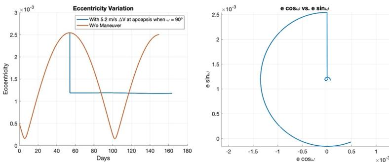
Figure 4: Results from the correction strategy. Left: eccentricity variation after maneuver. Right:  $e \cos(w) \times e \sin(w)$  transitioning to nearly frozen orbit.
