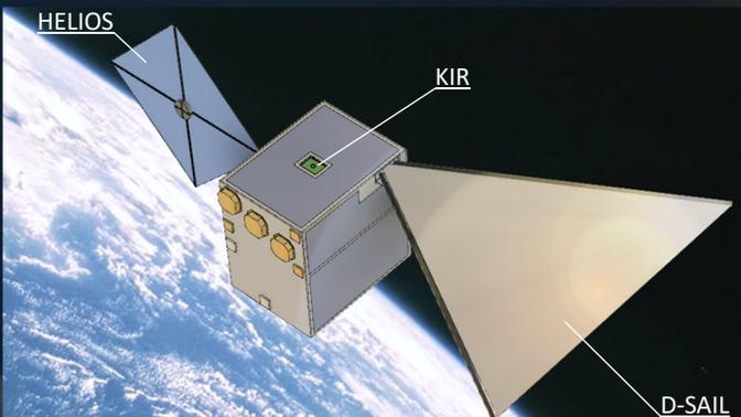
KIR: On-Orbit Demonstration of Micro-propulsion System using Water Propellant
