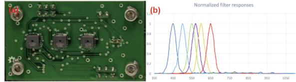
**Figure 2: (a) IS0 Pico SIM Payload Board, (b) Normalised Filter response of Payload Board**
