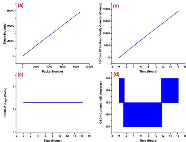
**Figure 8: (a) RTC value (seconds), (b) SD card write-read-verify counter, (c) C&DH Voltage (d) C&DH Current**
