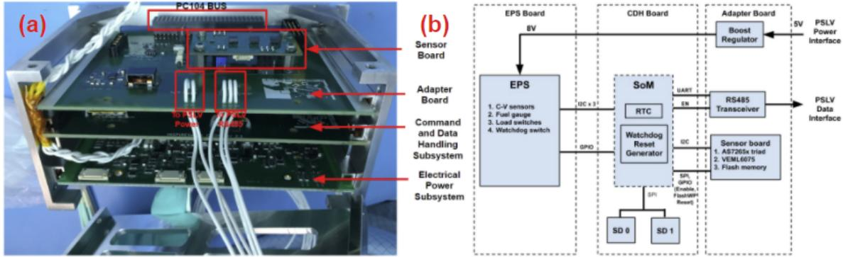
Figure 3: (a) IS0 Flight Model Assembly, (b) IS0 Block Diagram
