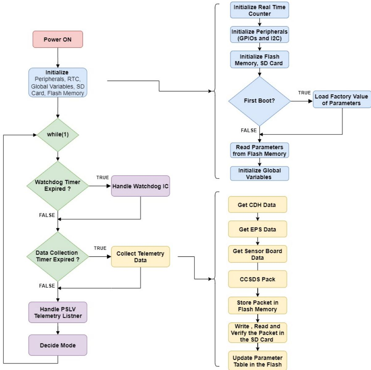
Figure 5: Flight Software Flowchart
