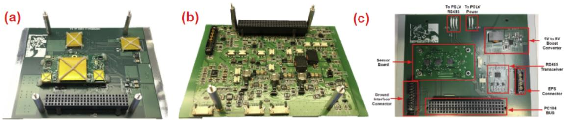
Figure 4: (a) IS0 CDH Board, (b)IS0 EPS Board, (c) IS-0 Adapter Board
