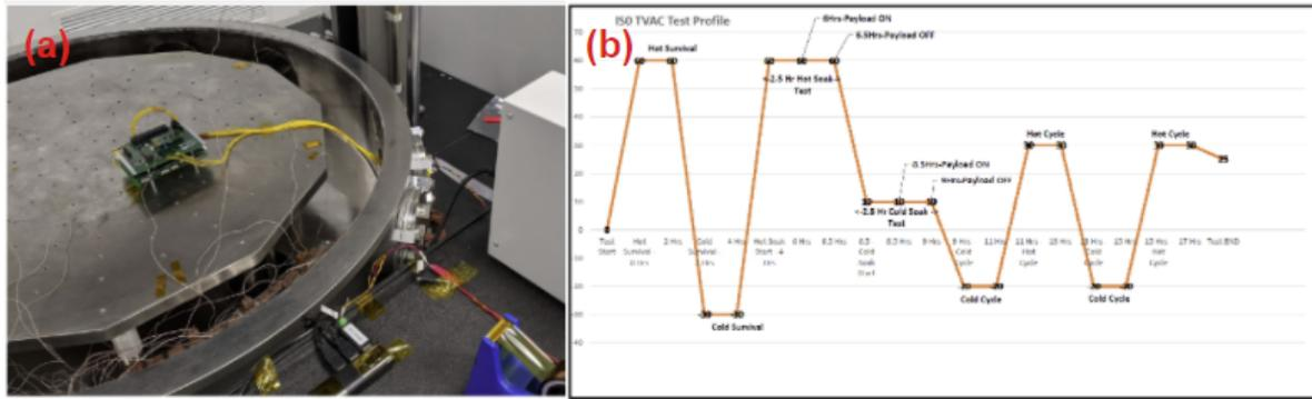
Figure 9: (a) ISO EM TVAC testing Setup, (b) TVAC Test Profile
