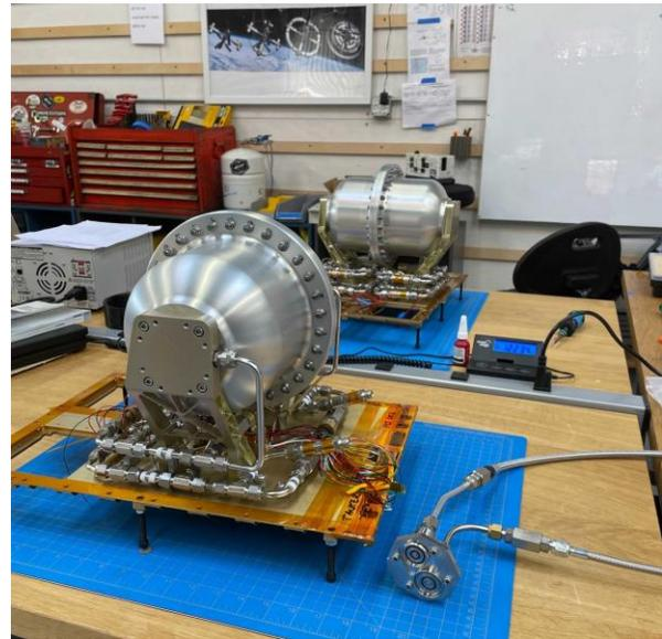
**Figure 6: The flight and flight spare primary refueling systems built up at Orbit Fab's facility. A RAFTI Block 1 Ground Coupling half can be seen in the bottom right.**
