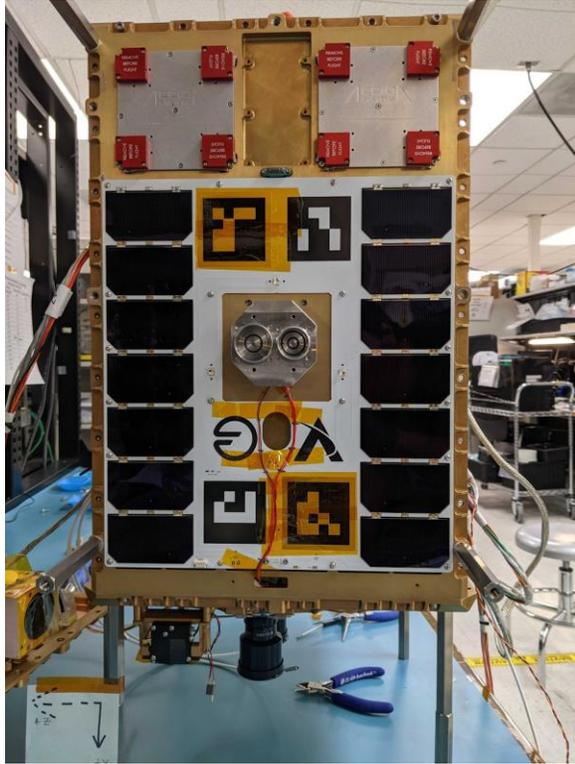
**Figure 8: Passive Spark embedded within an Astro Digital smart panel and installed on Tenzing for flight. Kapton tape will be removed before flight**
