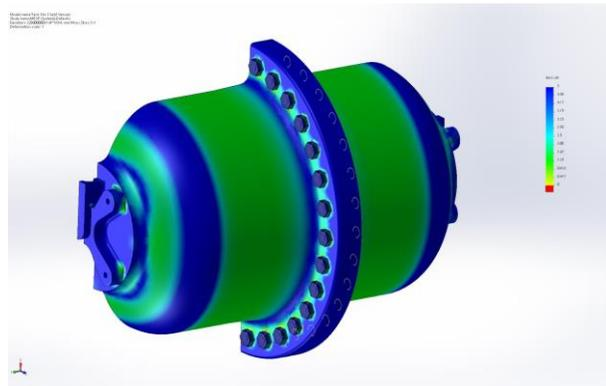
**Figure 5: Results from a stress analysis of the primary payload tank**
