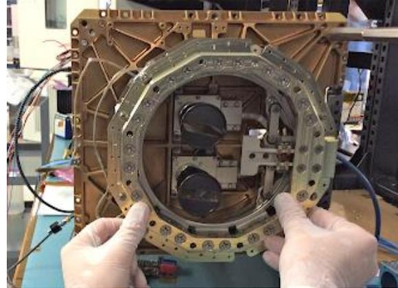
**Figure 9: SCOUT-Vision System installed on the Tenzing spacecraft**
