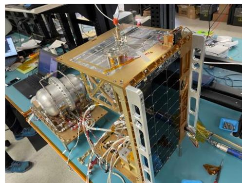
**Figure 7: The Halcyon and Primary refueling tank during integration with Tenzing and software checkout.**
