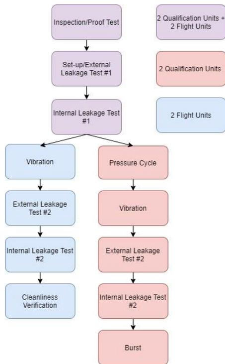
**Figure 6: A flow diagram of the qualification and acceptance testing campaigns**
