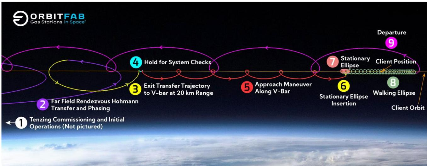
Figure 11: Notional Tenzing flyby trajectory in client-centric coordinate frame.
