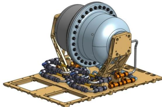
**Figure 4: CAD render of the primary payload mounted to a structural panel**
