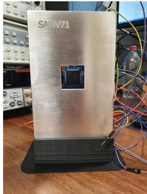
**Figure 3: SAMV71 behind an aluminium shield**
