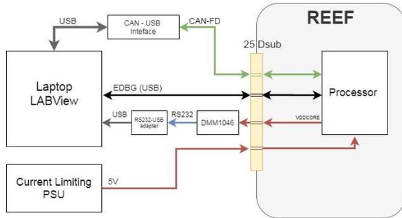
**Figure 6: REEF Test rig setup**
